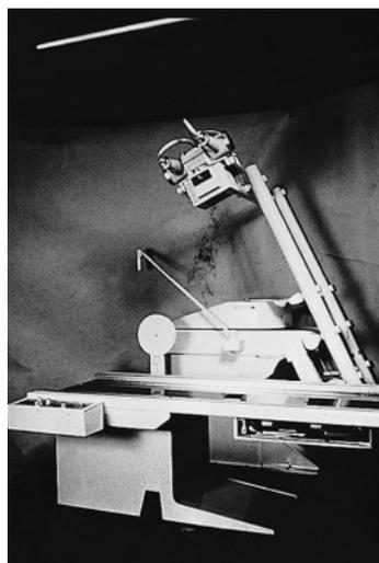
Figure 1. Overall view of the tomography system (Model LGM-1, Toshiba).
