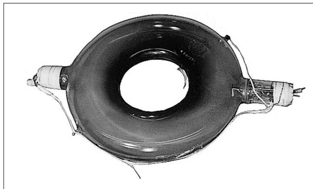
Figure 4. Doughnut tube for the 15-MeV betatron
