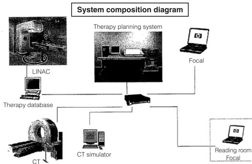
Figure 10. Typical example of radiotherapy system
