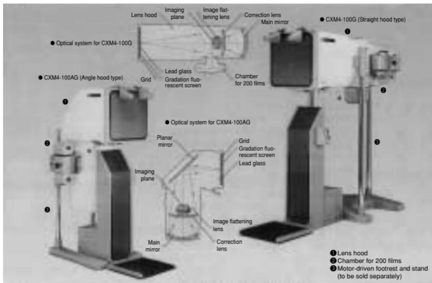
Figure 3. Structure of the mirror camera (reprinted from the catalog)
